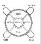
1 Press the MENU button and VOL+/VOL- button , till the **PIC** menu shown on the right display on the screen.
